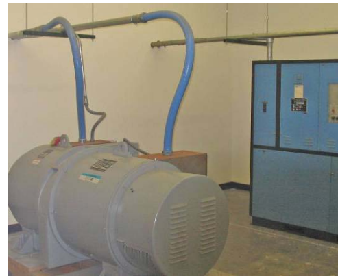
Variable frequency generators allow excitation tests up to 400 Hz
