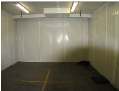
Anechoic chamber for accurate audible noise testing
